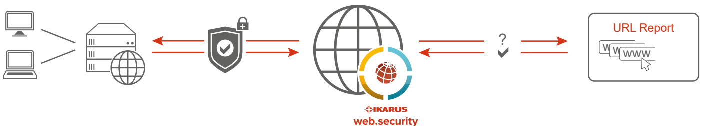
Fig. 1 - Central security proxy with reliable malware detection, flexible filter options and global URL category lists.
